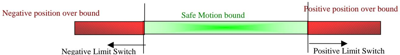
**Fig. 7-1 Definition of Motion bound of Specified Axis**
